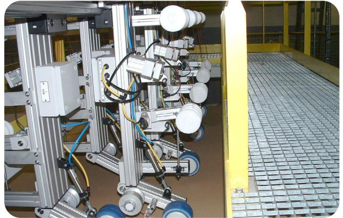
The PRS350 is a custom built, semi automatic system for applying Rippatape® to carton packaging. Sited between the rotary shear and slitter scorer, the integrated design comprises a platform and multiple application heads. The system is ideally suited to high volume users of Rippatape®.
